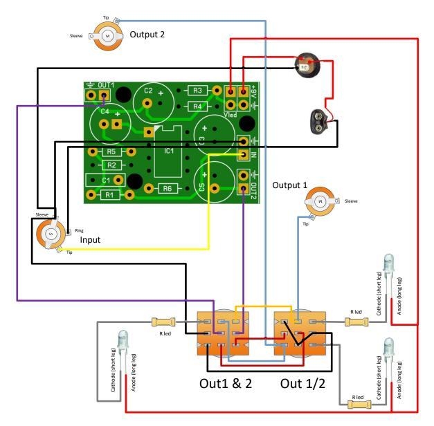
This is a beast to wire but works beautifully. You can either use 2 LED's for the "Out1 or Out2" switch or a bi-color LED to save space. When you switch the "Out1 and Out2" switch on it will turn off the "Out1 or Out2" LED to make sure you know which setting you are using.
