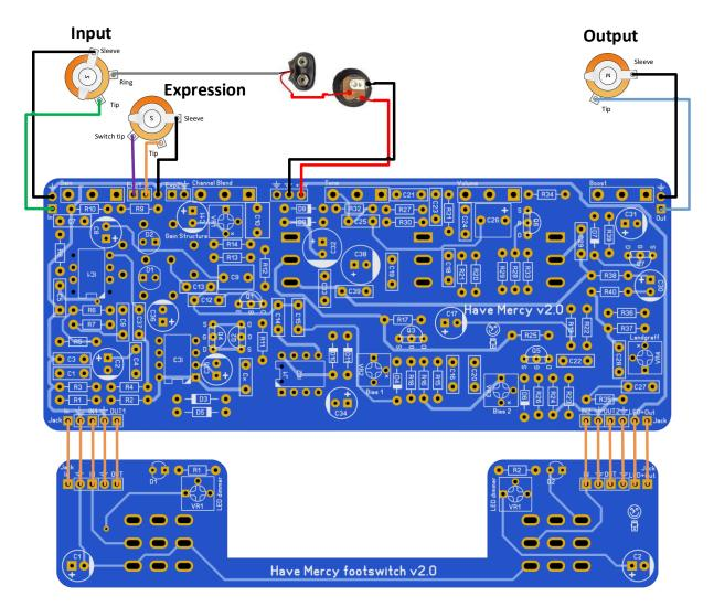
The footswitch PCB requires 2x 3PDT footswitches (**SW1** and **SW2**), 2x 390R resistors (**R1** and **R2**), 2x 3mm led of your choice for the status indicators (**D1** and **D2**), 2x 10uF caps (10V+) (**C1** and **C2**) and 2x 10k trimpots (**VR1** and **VR2**). All required parts are included in the BoM.
