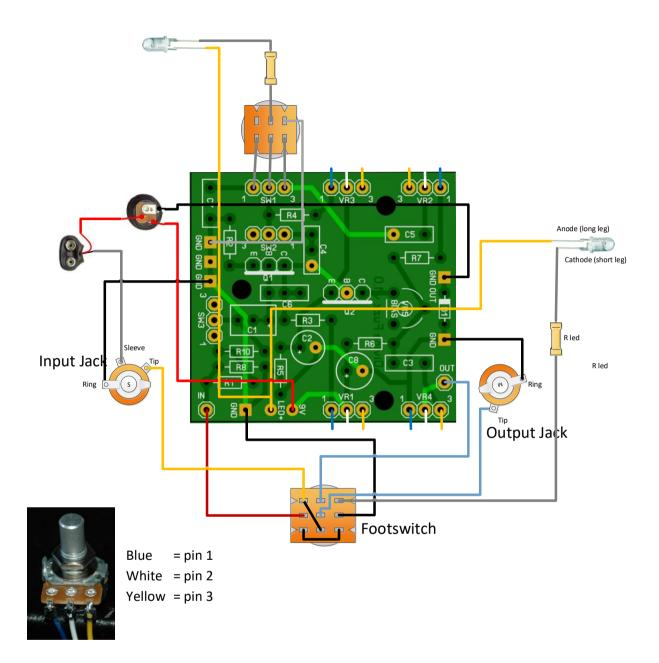
NB. If you do not want to use the D1 diode than remember to short it by soldering a lead instead.
