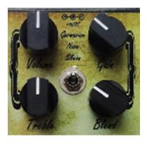
In the **Les Boutiques** effect the pot is split into separate Gain and Blend. You can now determine in every Gain setting how much of the clean signal you want to let bleed through. If you turn the Blend knob to the same position as the Gain knob, it will act as the Gain knob on the original.
