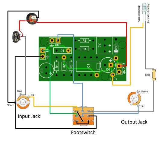
**R led** can be 3k3 or higher depending on your taste. Note that this wiring is based on star wiring and requires that the output jack is making good electrical contact with the enclosure. When testing is outside the enclosure please make sure you connect the output sleeve to ground!!
