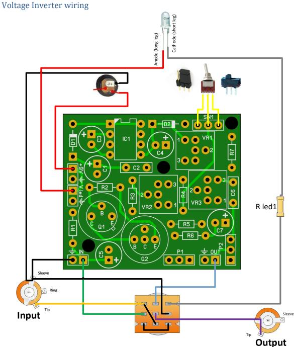
Note that **R led1** is **4k7** resistors. You can change this value depending on the type of LED you use but 4k7 is safe enough for almost all LEDs for (-)9V.
