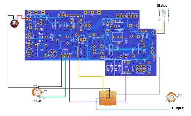
There is no wire from the output sleeve to ground so make sure there is good electrical contact between the jack and the enclosure, else you will need to solder a wire from the output sleeve to the input sleeve. The footswitch needs to have the missing output mixer resistors fitted directly on the switch like this:
