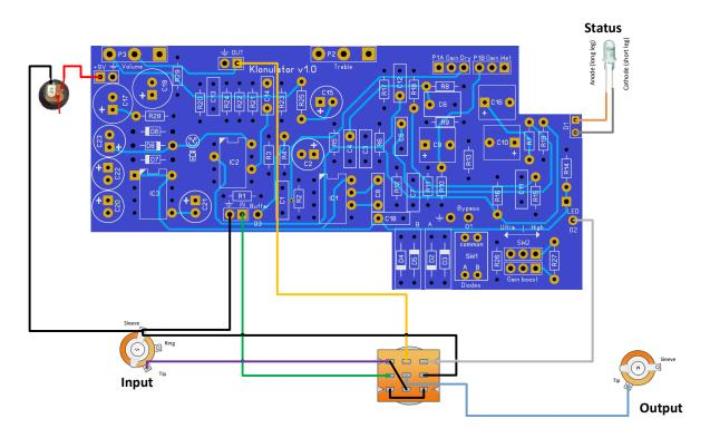
There is no wire from the output sleeve to ground so make sure there is good electrical contact between the jack and the enclosure, else you will need to solder a wire from the output sleeve to the input sleeve. The footswitch needs to have the 100k resistors fitted directly on the switch like this:
