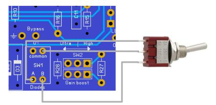
Or as a DP3T On/Z/On switch so you can also switch all diodes on (but not off!) Test the pole that are active in the middle position before you solder it.
