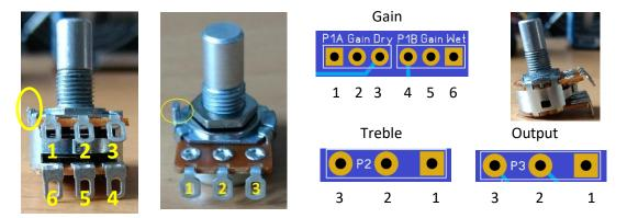
The wiring for the switches is the same, marking position 1 with a rectangle pad. It is a good idea to angle the top row of pins of the stereo pot about 45 degrees. This will give you a better fit for attaching the wires (top right picture).
