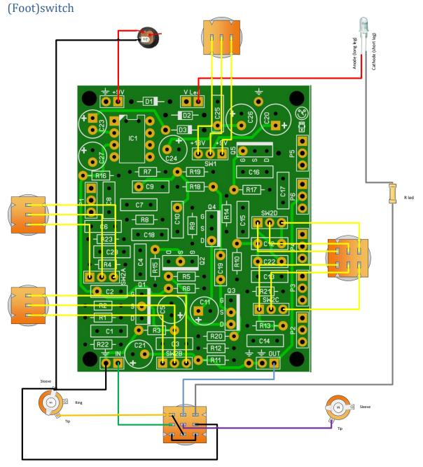
Note that this wiring is using a sort of star grounding and the output connector must make good electrical contact with the enclosure else the grounding will not work properly and the effect might start to buzz loudly.
