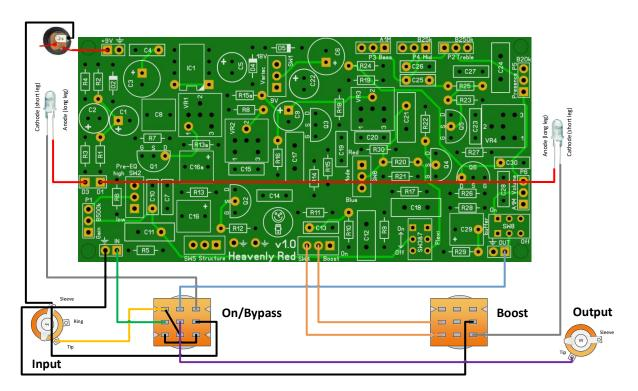
The LED switching is made as described by AMZ's anti Led pop setup. No need for an external LED current limiting resistor. **Keep cables as short as possible to prevent interference!**
