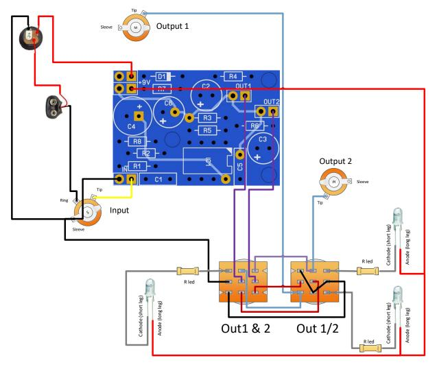
This is a beast to wire but works beautifully. You can either use 2 LED's for the "Out1 or Out2" switch or a bi-color LED to save space. When you switch the "Out1 and Out2" switch on it will turn off the "Out1 or Out2" LED to make sure you know which setting you are using.
