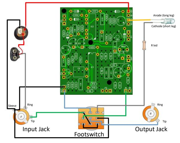
Note that **R led** is a **4k7** resistors. You can change this value depending on the type of LED you use but 4k7 is safe enough for almost all LEDs @ 9V.
