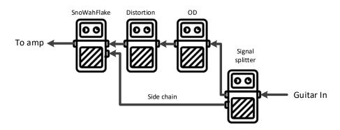
As mentioned before, if you do not want the effect to be used with side chaining then short both pads of **SW1** with a piece of lead wire (left over from eg. a resistor) else you can wire it as follows:
