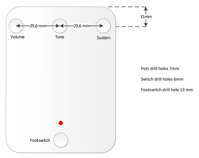
After you drilled the enclosure you can insert the potentiometers and attach them firmly to the enclosure. Now insert the PCB on the pots and if all fits ok you can solder the potentiometers to the PCB.
