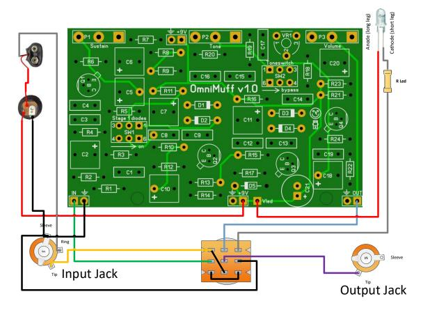
Note that **R led** is a **3k3/4k7** resistors. You can change this value depending on the type of LED you use but 3k3 is safe enough for almost all LEDs @ 9V.
