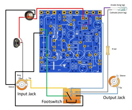
The LED requires a resistor (R led in the diagram) depending on the type of LED you are using. An ultra-bright red, green or blue LED requires a 4k7 resistor, diffuse green requires 680R. If you want to be more exact then go here: <u>http://www.muzique.com/schem/led.htm</u>
