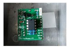
5. Now gently pull the board with switch out, making sure the LED sticks to the tape.
