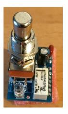
9. Make sure you screw the switch tightly to the enclosure and if all fits well, you can solder the LED to the PCB. I advise you to uninstall the PCB/switch for the off board wiring.
