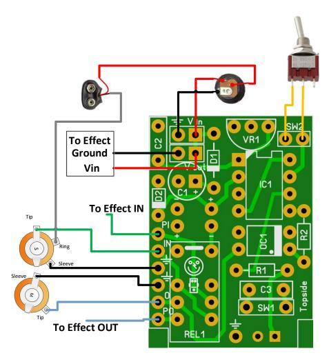
As you might have noticed in the diagram: Green means input and Blue means output.
