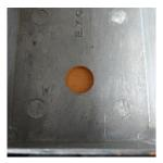
2. Stick some double sided tape to the right of the hole and remove the sticker revealing the sticky side.
