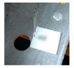
6. Press down on the led making sure not to damage it, but still hard enough to leave a mark in the tape. Remove the LED and mark that dent with a sharpie.
