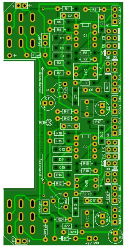
**NB.** There are some mistakes made in the channel and LED descriptions on the PCB. Green channel on the PCB should be *Red channel*, Red Channel on the PCB should be *Orange channel*. Led Green should be *Led Orange*. This does not affect the functioning of the board in any way, just read the instructions carefully!!
