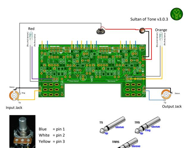
The wiring diagram is a copy of the latest original version. You should use a **RED LED** in the slots of **Led Red** in the (R Led=3k3 for 9V/18V) and an **ORANGE LED** in the **Led Green** (R Led=3k3 for 9V/18V).
