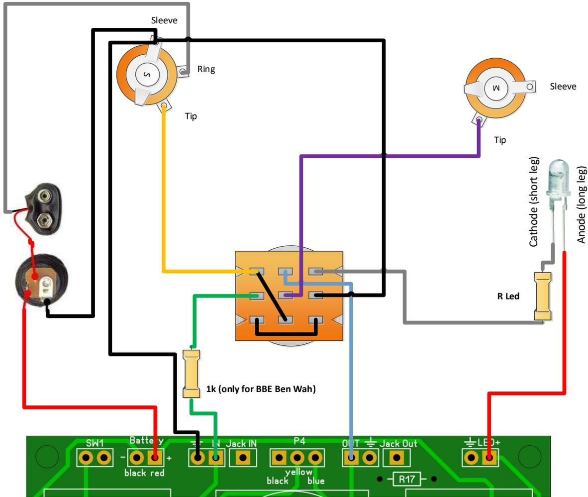
As the onboard DC jack is not installed, you will need to connect 2 DC pins on the board like this:
