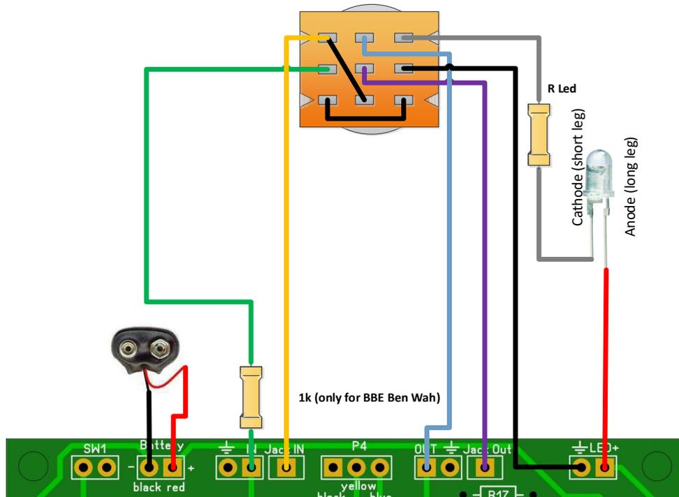
In this case you will need to populate **DC1**, **CONN IN** and **CONN OUT** with PCB mounted jacks. Note that **R led** is a **4k7** resistor. You can change this value depending on the type of LED you use but 4k7 is safe enough for almost all LEDs @ 9V.
