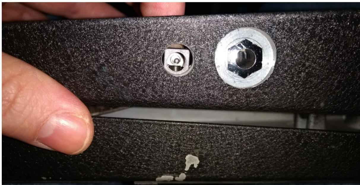
You can either use a plastic washer under the PCB or you can solder the DC jack with a small gap between the PCB and the jack. To check this, insert the DC jack in the DC input and determine the gap height. Make sure there is no pressure on the DC jack after inserting the jack!
