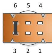
Also note that if you are not planning of implementing the buffer then you should leave out the parts and switch but short **pad 2 (SW2A)** and **pad 5 (SW2B)** on the PCB (also noted in the configuration sheet) else you will get NO SOUND!
