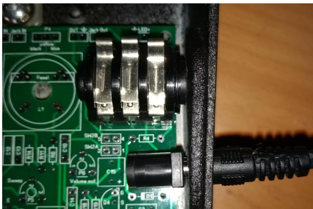
PS. It is always good to check that none of components or bottom of the PCB touch the enclosure. If you are unsure or parts are touching the enclosure, you could use some tape to prevent shortcuts.
