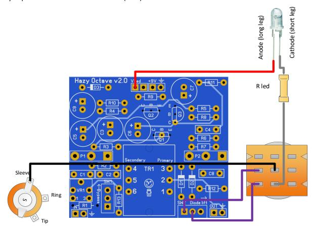
Also note that if you do not want to use the diode lift switch (**SW2**) then jumper the middle pad of **SW2** to the rectangle pad with a spare piece of wire (eg from a resistor).
