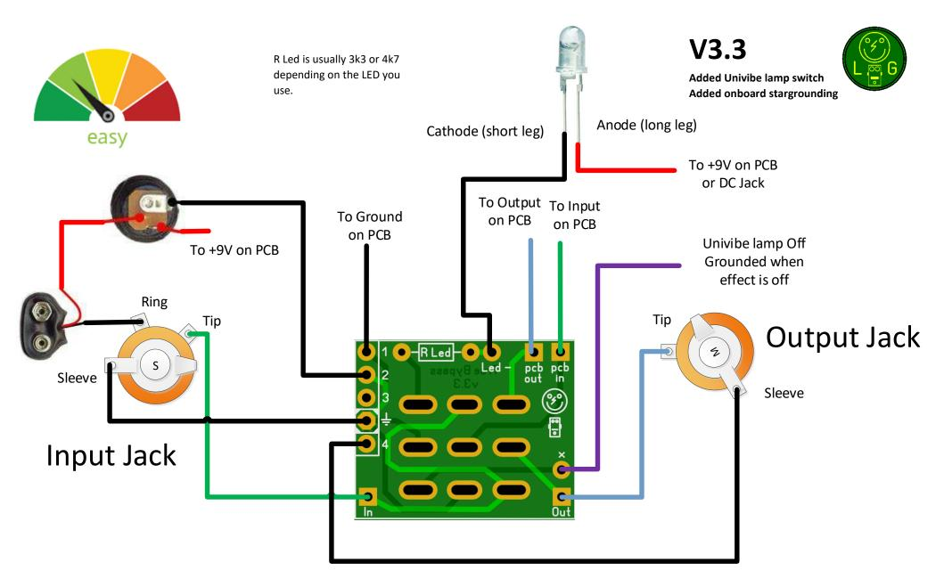
When patching 2 effects together then connect <u>Out from effect A</u> to <u>In from effect B</u>.
