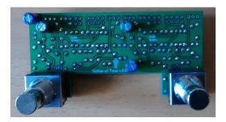
Finally solder the presence/treble boost trim pots **VR1** and **VR2**. If you want to control the presence externally then do not solder **VR1** and **VR2** but use B50k Alpha 16mm pots. For your convenience I marked the pinning on the PCB. The pots default setting is <u>all the way to the right</u>. To boost treble, turn the pots to the left.
