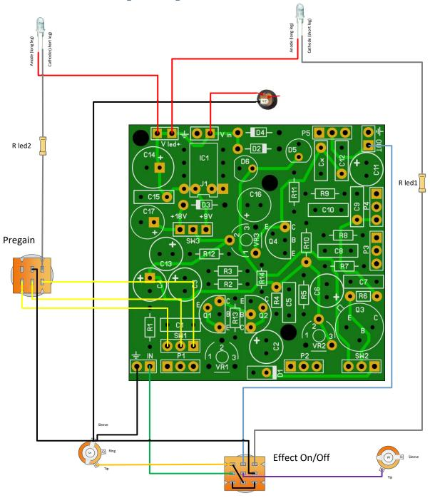
Note that **R led1 and R led2** are **4k7** resistors. You can change this value depending on the type of LED you use but 4k7 is safe enough for almost all LEDs for both 9V as 18V.
