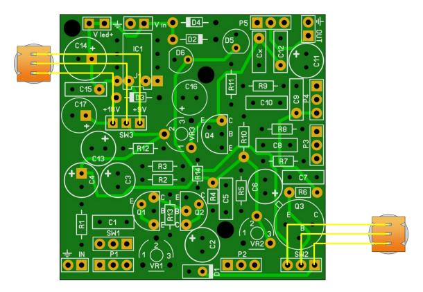
\* The Throbak uses an internal trimpot for the pre-gain. If you do not want an extra external pot you can substitute the P1 Alpha pot for a internal trimpot (Bourns 3296W style)
