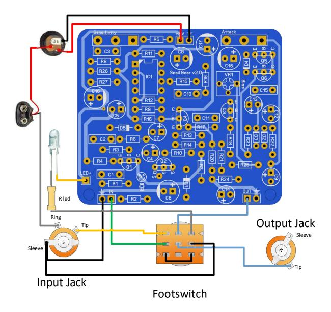
The LEDs requires a resistor (R led in the diagram) depending on the type of LED you are using. To be safe use a 3k3 or 4k7 resistor. If you want to be more exact then go here: <a href="http://www.muzique.com/schem/led.htm">http://www.muzique.com/schem/led.htm</a>
