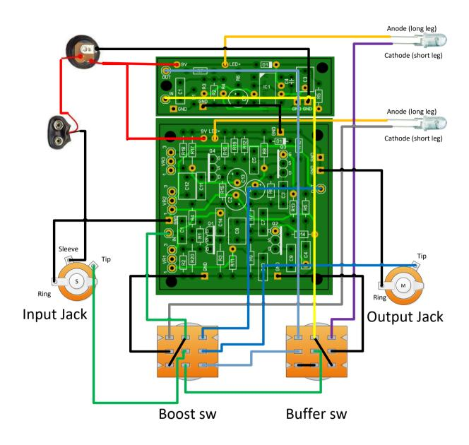
When the buffer switch is **DOWN**, the buffer is **ON** when the boost is **OFF**.
