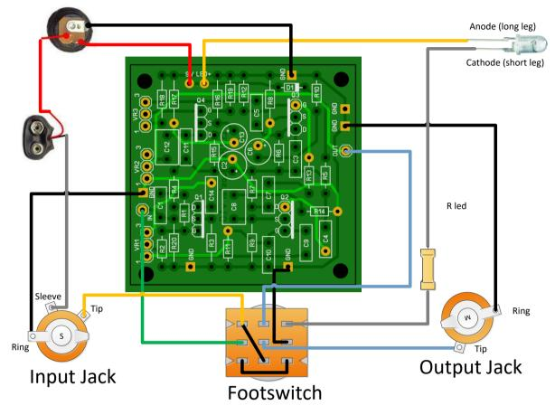
Notice that in the "off" position the effect input is connected to ground to prevent possible oscillation.
