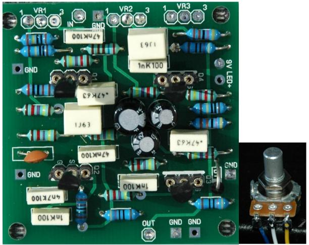
On the picture of the pot you can make out the pin sequence on the board.
