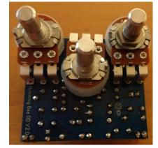
Insert the potentiometers in the holes of the enclosure and attach the PCB. Note that the PCB mount potentiometers will be attached on the back of the PCB. When everything fits ok, solder the potentiometers to the PCB.
