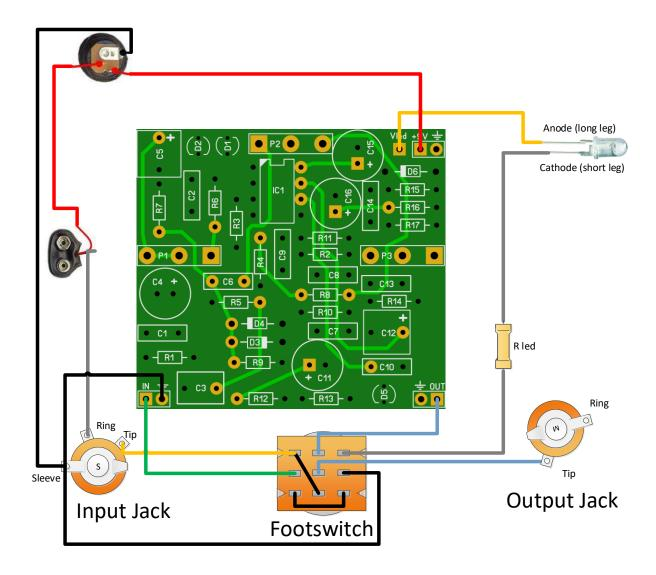
Notice that in the "off" position the effect input is connected to ground to prevent possible oscillation. The diagram is also based on star wiring where all ground connections go to the sleeve of the input jack.
